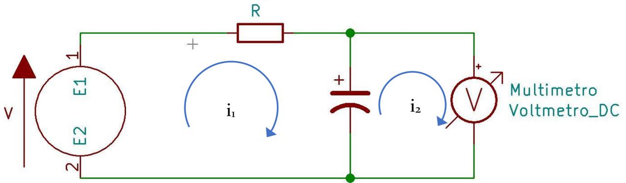
$$\begin{cases} V = Ri_1 + \frac{1}{C} \int_0^t i_1 dt + V(0) \\ 0 = \frac{1}{C} \int_0^t i_2 dt + V(0) + R_V i_2 \end{cases}$$
